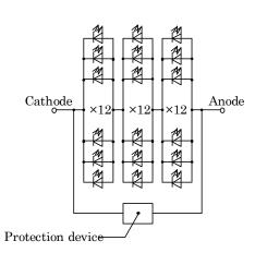
It has a protection device built in as a protection circuit against static electricity.
