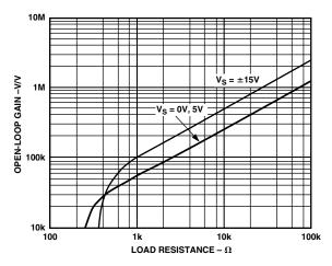
TPC 7. Open-Loop Gain vs. Load Resistance
