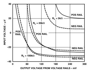
TPC 10. Input Error Voltage with Output Voltage within 300 mV of Either Supply Rail for Various Resistive Loads;  $V_S = \pm 5 \text{ V}$
