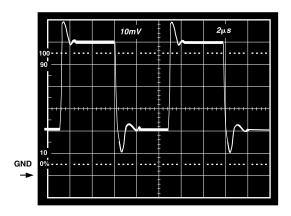
Figure 12.  $V_S = 5 V$ , 0 V; Unity Gain Follower Response to 40 mV Step Centered 40 mV above Ground
