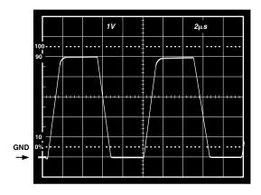
Figure 11.  $V_S = 5 V$ , 0 V; Gain-of-Two Inverter Response to 2.5 V Step Centered –1.25 V below Ground
