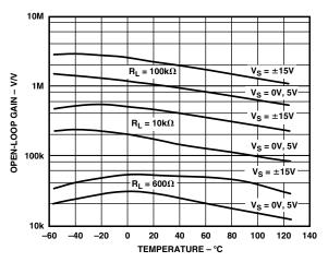
TPC 8. Open-Loop Gain vs. Temperature
