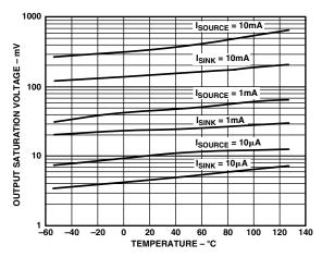
TPC 19. Output Saturation Voltage vs. Temperature
