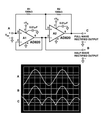
Figure 20. Single Supply Half- and Full-Wave Rectifier
