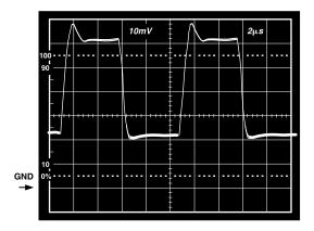
Figure 13.  $V_S = 5 V$ , 0 V; Gain-of-Two Inverter Response to 20 mV Step, Centered 20 mV below Ground
