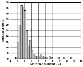
Figure 1. Typical Distribution of Input Bias Current
