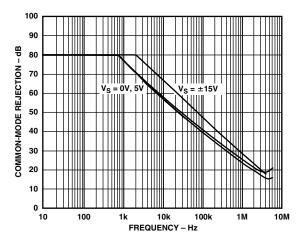
TPC 16. Common-Mode Rejection vs. Frequency
