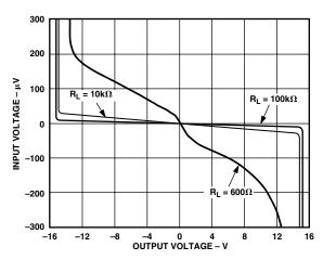
TPC 9. Input Error Voltage vs. Output Voltage for Resistive Loads
