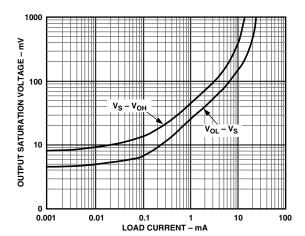
TPC 18. Output Saturation Voltage vs. Load Current
