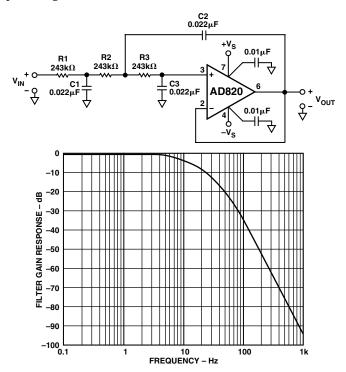
Figure 22. 10 Hz Sallen Key Low-Pass Filter
