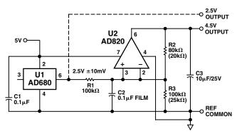
Figure 21. Single Supply 4.5 V Low Dropout Reference
