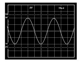
Figure 4. 20 V, 25 kHz Sine Input; Unity Gain Follower;  $R_L = 600~\Omega,~V_S = \pm\,15~V$
