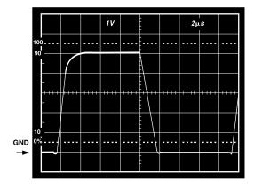
Figure 8.  $V_S = 5 V$ , 0 V; Unity Gain Follower Response to 0 V to 5 V Step
