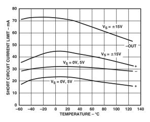
TPC 20. Short Circuit Current Limit vs. Temperature
