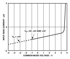
TPC 4. Input Bias Current vs. Common-Mode Voltage;  $V_S = +5 V$ , 0 V and  $V_S = \pm 5 V$
