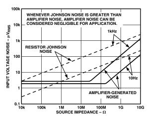
Figure 15. Total Noise vs. Source Impedance
