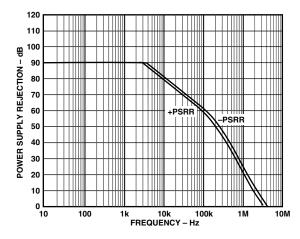
TPC 22. Power Supply Rejection vs. Frequency
