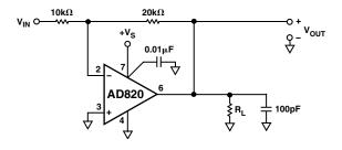
Figure 10. Gain of Two Inverter
