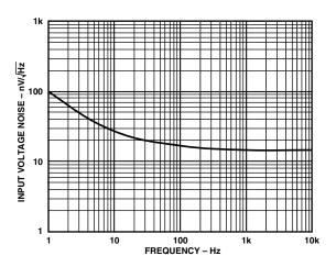
TPC 11. Input Voltage Noise vs. Frequency
