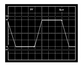
Figure 6. Large Signal Response Unity Gain Follower;  $V_S = \pm 15~V,~R_L = 10~k\Omega$
