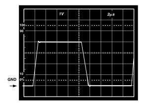
Figure 5.  $V_S = 5 V$ , 0 V; Unity Gain Follower Response to 0 V to 4 V Step
