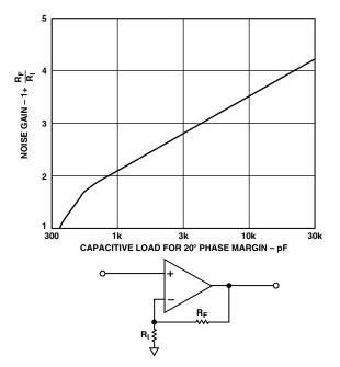
Figure 17. Capacitive Load Tolerance vs. Noise Gain
