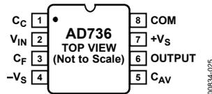
Figure 2. Pin Configuration
