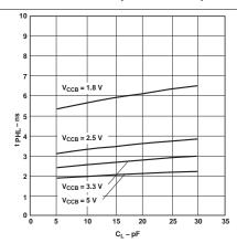
Figure 13. Typical Propagation Delay of High-to-Low (A to B) vs Load Capacitance  $T_A = 25$ °C,  $V_{CCA} = 5$  V
