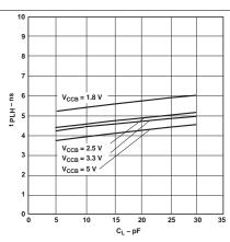
Figure 8. Typical Propagation Delay of Low-to-High (B to A) vs Load Capacitance  $T_A = 25^{\circ}C$ ,  $V_{CCA} = 2.5$  V
