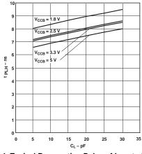
Figure 4. Typical Propagation Delay of Low-to-High (B to A) vs Load Capacitance  $T_A = 25^{\circ}C$ ,  $V_{CCA} = 1.8 \text{ V}$
