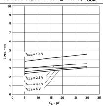
Figure 11. Typical Propagation Delay of High-to-Low (B to A) vs Load Capacitance  $T_A = 25^{\circ}C$ ,  $V_{CCA} = 3.3 \text{ V}$
