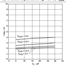
Figure 15. Typical Propagation Delay of High-to-Low (B to A) vs Load Capacitance  $T_A$  = 25°C,  $V_{CCA}$  = 5 V
