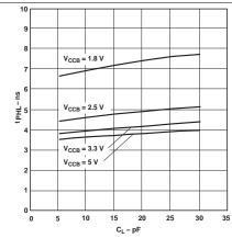
Figure 1. Typical Propagation Delay of High-to-Low (A to B) vs Load Capacitance  $T_A = 25^{\circ}C$ ,  $V_{CCA} = 1.8 \text{ V}$
