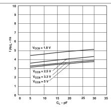
Figure 7. Typical Propagation Delay of High-to-Low (B to A) vs Load Capacitance  $T_A = 25^{\circ}C$ ,  $V_{CCA} = 2.5 \text{ V}$
