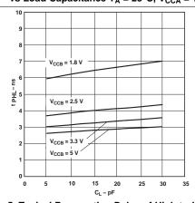
Figure 5. Typical Propagation Delay of High-to-Low (A to B) vs Load Capacitance  $T_A = 25^{\circ}C$ ,  $V_{CCA} = 2.5 \text{ V}$
