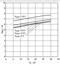
Figure 3. Typical Propagation Delay of High-to-Low (B to A) vs Load Capacitance  $T_A = 25^{\circ}C$ ,  $V_{CCA} = 1.8 \text{ V}$
