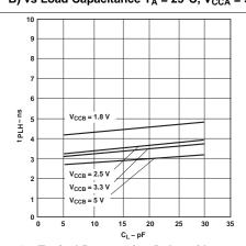
Figure 12. Typical Propagation Delay of Low-to-High (B to A) vs Load Capacitance  $T_A = 25^{\circ}C$ ,  $V_{CCA} = 3.3 \text{ V}$
