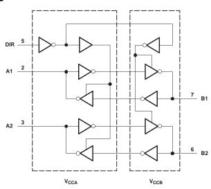
Figure 18. Logic Diagram (Positive Logic)
