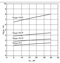
Figure 14. Typical Propagation Delay of Low-to-High (A to B) vs Load Capacitance  $T_A = 25^{\circ}C$ ,  $V_{CCA} = 5 \text{ V}$
