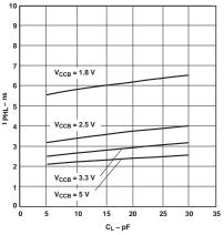
Figure 9. Typical Propagation Delay of High-to-Low (A to B) vs Load Capacitance  $T_A = 25^{\circ}C$ ,  $V_{CCA} = 3.3 \text{ V}$
