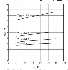
Figure 6. Typical Propagation Delay of Low-to-High (A to B) vs Load Capacitance  $T_A = 25^{\circ}C$ ,  $V_{CCA} = 2.5$  V
