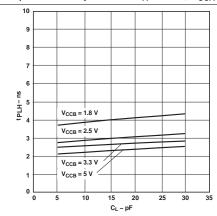
Figure 16. Typical Propagation Delay of Low-to-High (B to A) vs Load Capacitance  $T_A = 25^{\circ}C$ ,  $V_{CCA} = 5$  V
