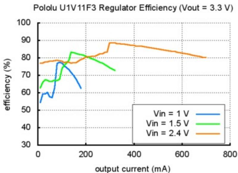
The maximum achievable output current is approximately proportional to the ratio of the input voltage to the output voltage. If the input current exceeds the switch current limit (typically somewhere between 1.2 and 1.5 A), the output voltage will begin to drop. Additionally, the
