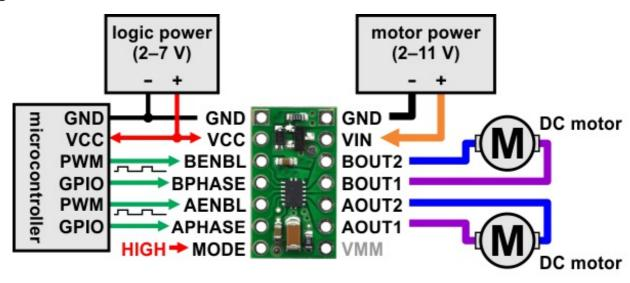
Minimal wiring diagram for connecting a microcontroller to a DRV8835 dual motor driver carrier in phase-enable mode.
