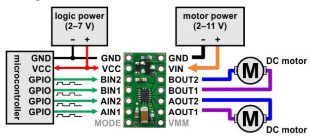
Minimal wiring diagram for connecting a microcontroller to a DRV8835 dual motor driver carrier in in-in mode.
