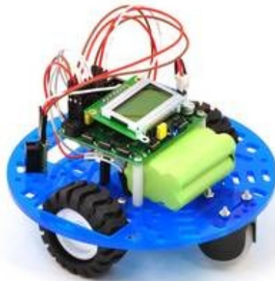
Pololu 5" round robot chassis RRC04A includes two spacers.
