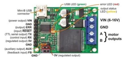
• Simple bidirectional control of one DC brush motor.
