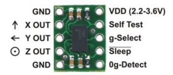
The board is powered by supplying 2.2 V to 3.6 V on the VDD pin. Note that this part does not have 5V-tolerant pins, so external components (such as voltage dividers) are required when interfacing the board's g-Select, Self Test, and Sleep pins with 5V systems. Connections to these pins are optional; the board will work with these pins disconnected as long as the sleep pin is driven high with an on-board solder bridge as described below.
