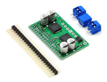
A 25-pin straight breakaway male header is included with the MC33926 dual carrier board, which can be used to connect the PCB to perfboards or breadboards. The board also includes three 2-pin 3.5mm terminal blocks for making simple motor connections.
