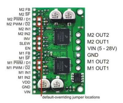
The default states of many of the MC33926 logic input pins requires that many external connections be made to use this board. To reduce the number of necessary external connections, the board has seven default-overriding jumpers. All of the default-overriding jumpers are tied to VDD, except the D1 jumpers, which are tied to GND. All VDD jumper pads are circles; the ground jumper pads are square. Note that the board has only one invert, slew, and enable pin; each of
