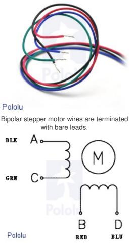
Bipolar stepper motor wiring diagram.
