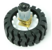
Pololu wheel 42×19mm with micro metal gearmotor.
