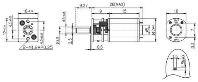
Micro metal gearmotor dimensions (units in mm).
