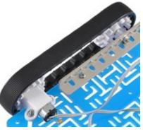
Pololu 30T track set with drive sprocket mounted on a micro metal gearmotor to the left; idler sprocket is on the right.
