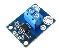
This board carries the Allegro's ACS714ELCTR-05B-T hall effect-based linear current sensor, which offers a low-resistance ( $\sim$ 1.2m $\Omega$ ) current path and electrical isolation up to 2.1kV RMS.
