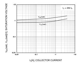
Figure 2. Base-Emitter Saturation Voltage Collector-Emitter Saturation Voltage
