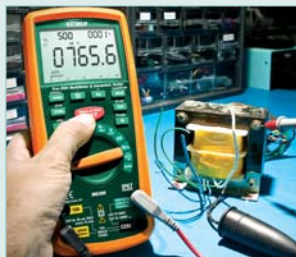
Measure the insulation resistance of transformer windings
