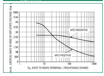
Figure 9. Critical Rate of Rise of Commutating Voltage
