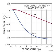
Figure 8. Ceramic Capacitor DC Bias Characteristics
