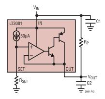
Figure 13. Reducing Power Dissipation Using a Parallel Resistor
