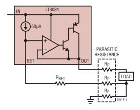
Figure 10. Connections for Best Load Regulation
