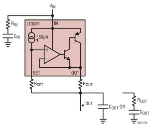
Figure 6. Input and/or Output Capacitors May Be Used for Compensation
