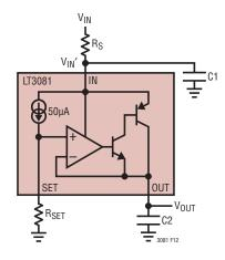
Figure 12. Reducing Power Dissipation Using a Series Resistor
