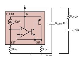
Figure 5. Compensation from Input to Output of Current Source Provides Stability
