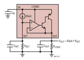
Figure 1. Basic Adjustable Regulator
