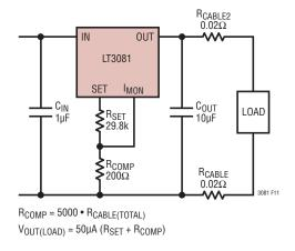
Figure 11. Using I<sub>MON</sub> to Compensate for Cable Drops
