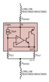
Figure 4. Adding Series Resistance Decouples and Dampens Long Line Reactances
