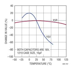
Figure 7. Ceramic Capacitor Temperature Characteristics
