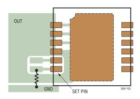
Figure 2. Guard Ring Layout Example of DF Package
