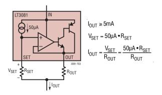
Figure 3. Using the LT3081 as a Current Source
