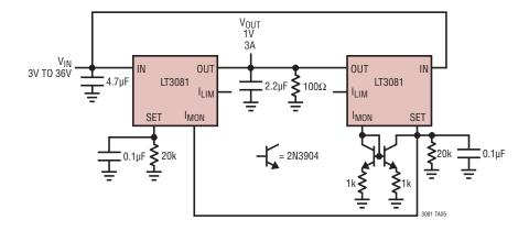
Constant-Voltage, Constant-Current 20V/3A Lab Supply
