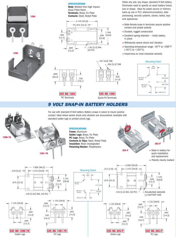
NOTE: For battery thicknesses under .640 (16.3); specify Cat. No. 1290 or 1291.
