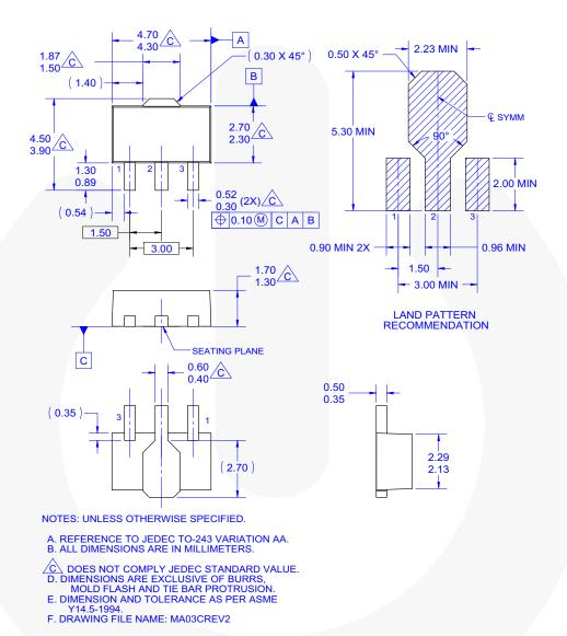
Figure 4. 3-Lead, SOT-89, JEDEC TO-243, Option AA
