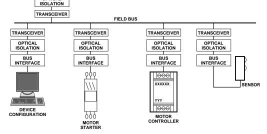
Figure 17. Typical Field Bus Communication Physical Model.
