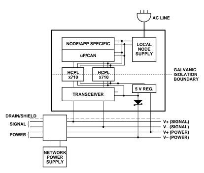
Figure 18. Typical DeviceNet Node.
