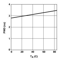
Figure 4. Typical Pulse Width
