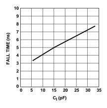
Figure 10. Typical Fall Time vs. Load Capacitance.
