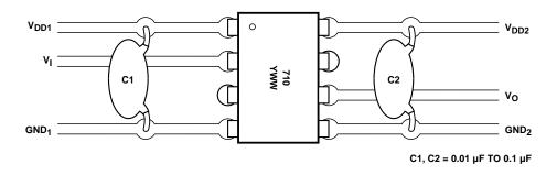
Figure 13. Recommended Printed Circuit Board Layout.
