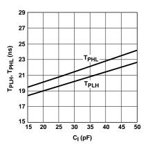
Figure 7. Typical Propagation Delays vs. Output Load Capacitance.
