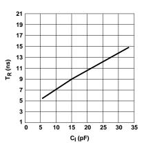
Figure 9. Typical Rise Time vs. Load Capacitance.
