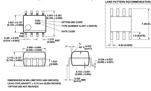
NOTE: FLOATING LEAD PROTRUSION IS 0.15 mm (6 mils) MAX.
