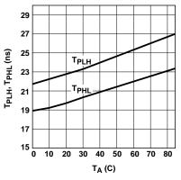
Figure 3. Typical Propagation Delays vs. Temperature.
