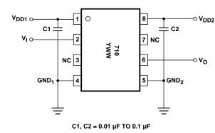
Figure 12. Recommended Printed Circuit Board Layout.
