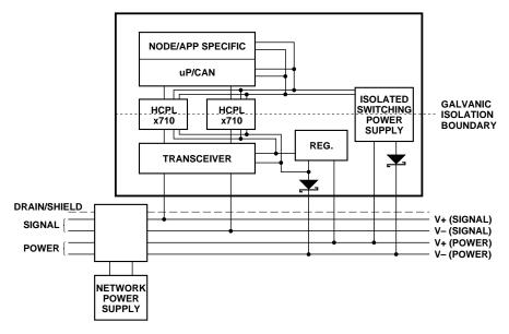
Figure 19. Isolated Node Powered by the Network.
