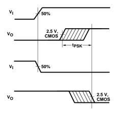
Figure 15. Propagation Delay Skew Waveform.
