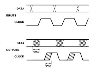
Figure 16. Parallel Data Transmission Example.
