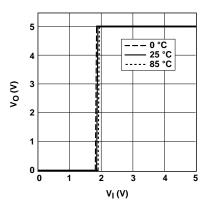
Figure 1. Typical Output Voltage vs. Input Voltage.
