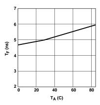
Figure 6. Typical Fall Time vs. Temperature.
