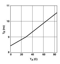
Figure 5. Typical Rise Time vs. Temperature.
