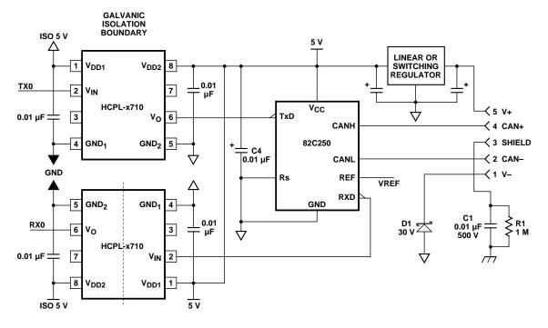
Figure 22. Recommended DeviceNet Application Circuit.
