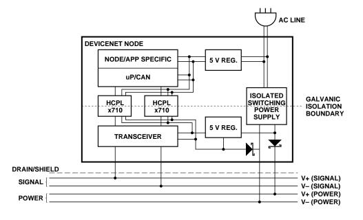
Figure 21. Isolated Node Providing Power to the Network.
