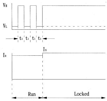
3rd wire signal Run : Square Wave Locked : V<sub>H</sub> or V<sub>L</sub>
