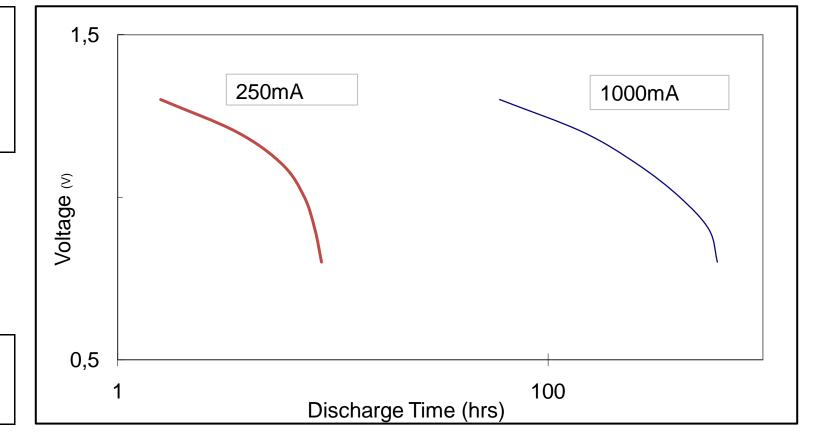
Test environment: 20  $^{\circ}$ C  $\pm$  2,60%  $\pm$  15% R.H, Load resistance: 3.9 ohms, time: 0.3s
