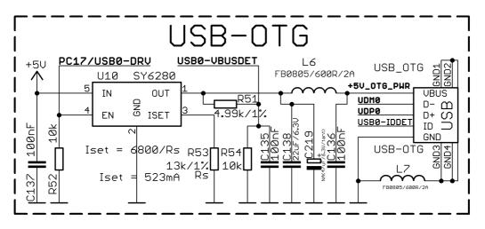
The USB\_OTG features Low Loss Power Distribution Switch SY6280 which protects the board in case the devices you have plugged to the USB\_OTG attempt to draw more current than 523mA combined. The maximum current available on the 5V USB\_OTG is exactly 523mA.
