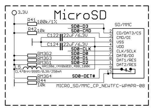
This slot is typically used for booting the OS, due to the larger capacities of the microSD cards (compared to SD or MMC cards). It is suggested to have an SD card with a proper Linux/Android image especially if you have ordered a version of the board without NAND memory. It is also recommended to use Class 10 (10MByte/sec) card for faster read/write operations, lower class cards (especially higher capacity ones) might slow down the whole system.
