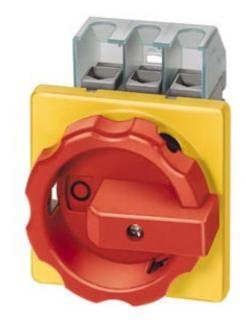
MAIN/EMERG. STOP SWITCH 3-POLE IU=25, P/AC-23A AT 400V=9.5KW FRONT MOUNTING FOUR-HOLE MOUNTING ROTARY ACTUATOR RED/YELLOW (EMERG. STOP)
